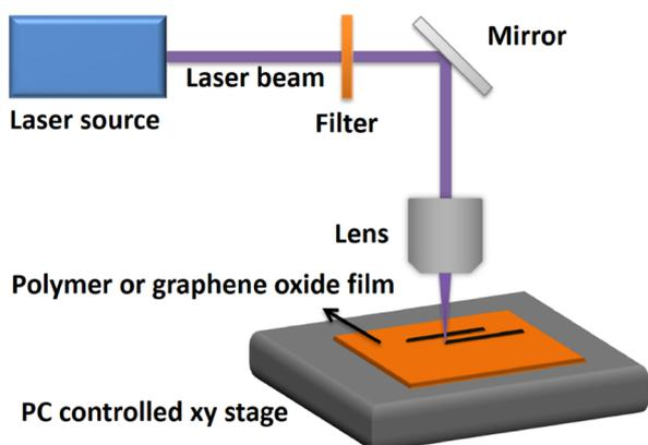
Figure 1. Schematic illustration of the laser direct writing system.
