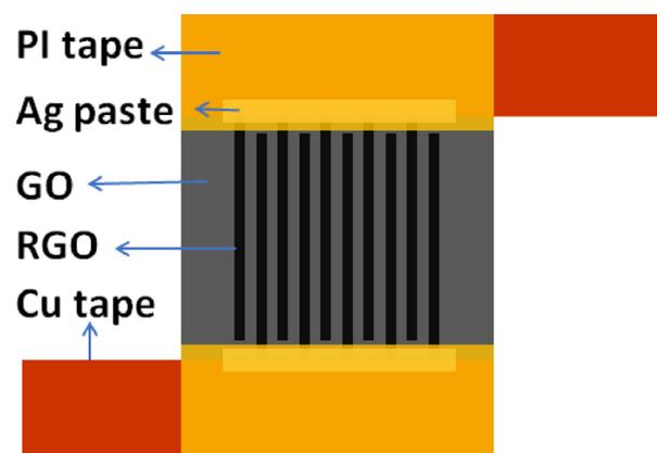
Figure 2. Schematic illustrating of a MSC device obtained by laser direct writing. Ag paste was used to make good connection between Cu tape electrodes and RGO lines.
