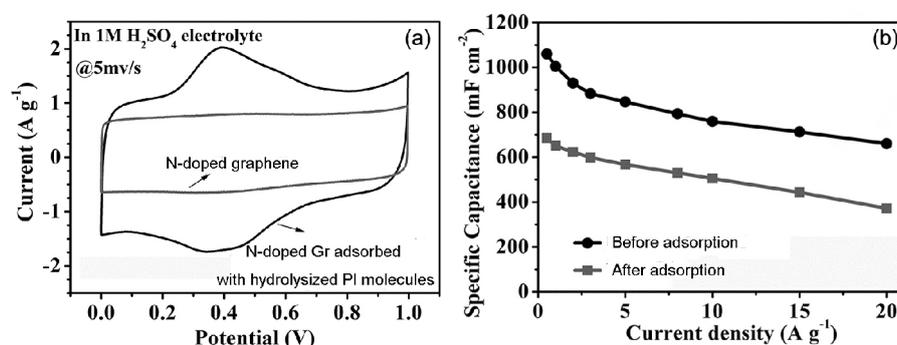
**Figure 1.** (a) Comparison to the electrochemical performance of N-doped graphene electrode before and after adsorption of hydrolyzed PI molecules. (a) CV curves. (b) Capacitance Vs. discharging current density in galvanostatic CD measurement.
