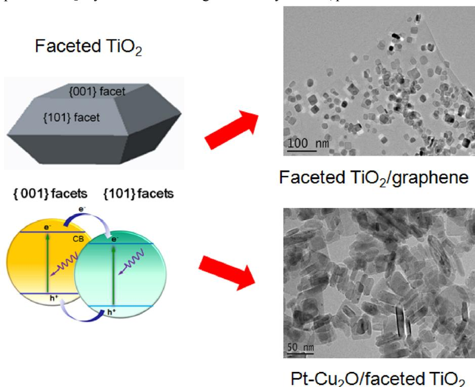
**Figure 1.** Schematic diagram of graphene and metal modified faceted TiO<sub>2</sub> nanocrystals.
