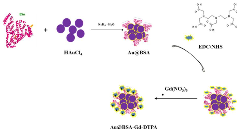
**Figure 1.** A schematic illustration of the preparation of the Au@BSA-Gd-DTPA.
