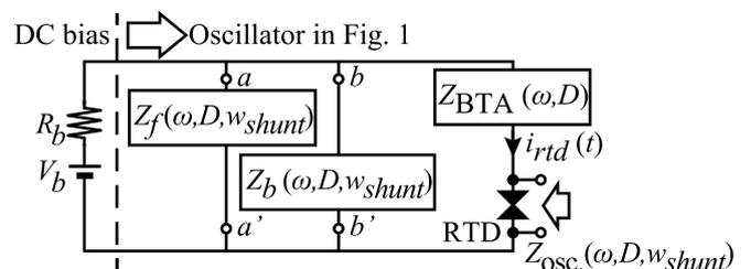
Figure 2 Block expressions of an equivalent circuit for the oscillator shown in Figure 1.
