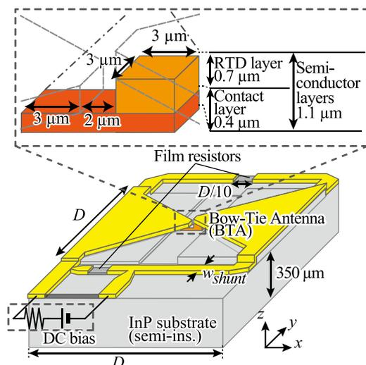
Figure 1 Schematics of a proposed oscillator.
