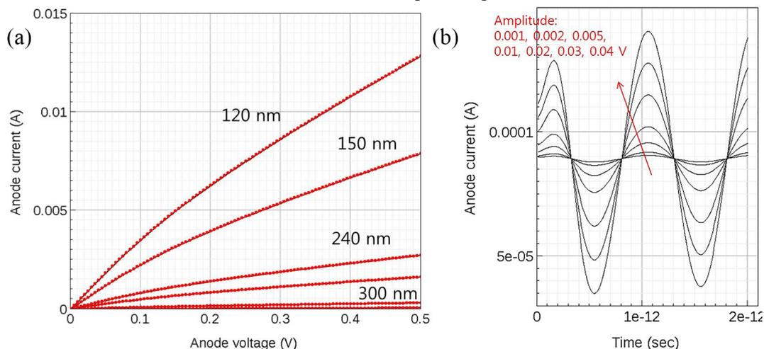
Figure 1 (a) DC IV characteristics of various  $N^+NN^+$  devices, which are obtained from the deterministic Boltzmann equation solver. (b) Transient results of an  $N^+NN^+$  device whose total length is 1200 nm. The DC bias voltage is 0.8 V. AC voltages of 1 THz with various amplitudes are applied to the anode terminal. The first two periods are simulated.
