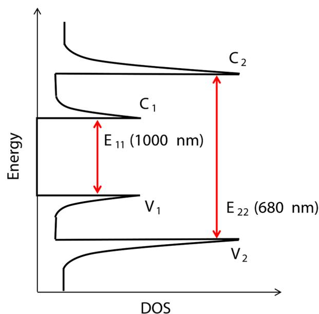
**Figure 1.** Electronic density of States (DOS) of (8,3) SWCNT.
