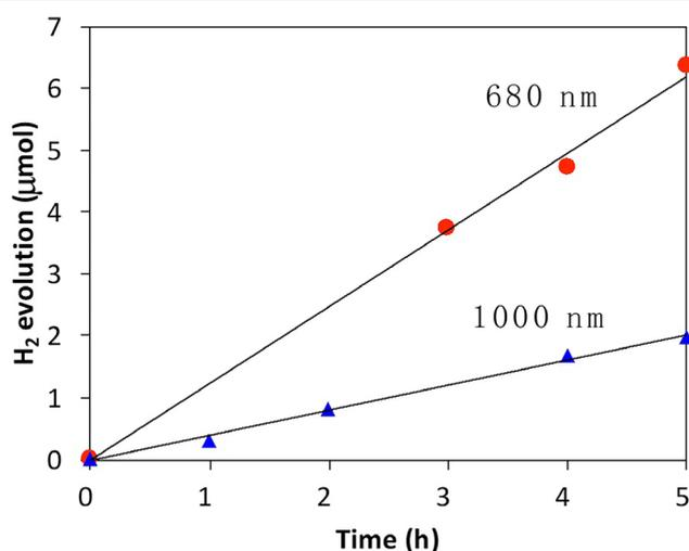
**Figure 4.** Time dependencies of Photocatalytic H<sub>2</sub> evolution from using SWCNT photocatalyst under monochromatic light at 680 nm (●) and 1000 nm (▲).
