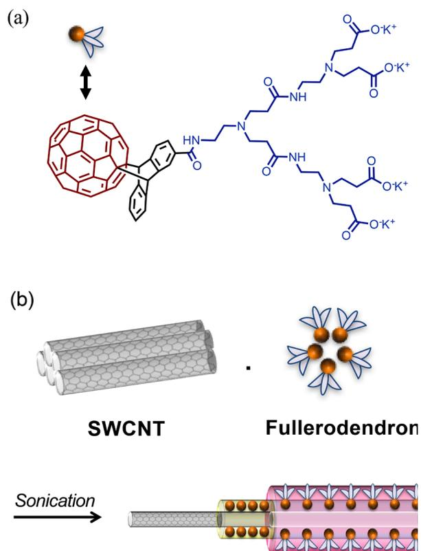
**Figure 2.** (a) Molecular structure of fullerodendron. (b) Schematic illustration of the fabrication of SWCNT/fullerodendron nano-hybrids (SWCNT photocatalysts).
